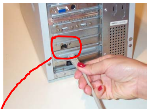
STEP 1 - Unplug the RJ45 Ethernet Cable that runs from the So-net's ADSL Modem
