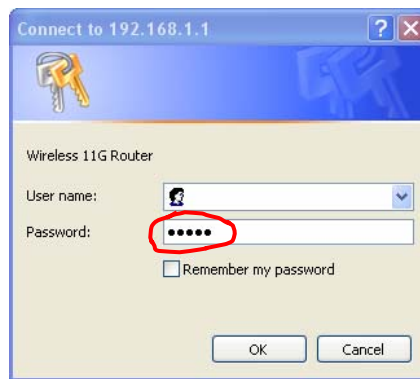
STEP 4 - When this screen pops up, skip the User name, enter your Password (default as "admin"), then press OK
