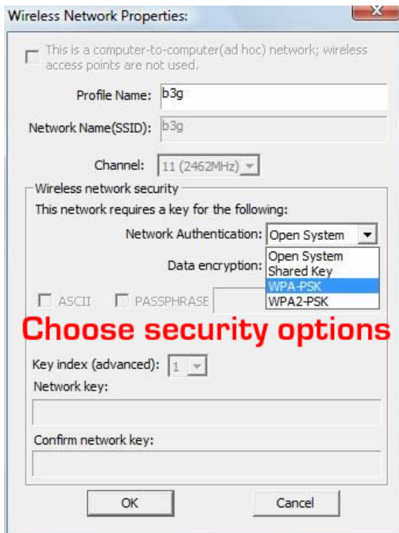
Figure 5 Set up the security option corresponding to the wireless router of SSD b3g
