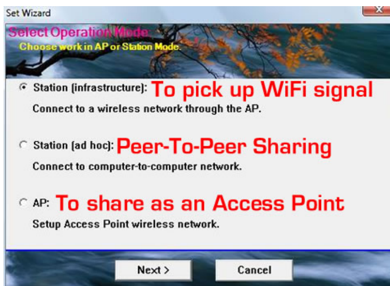
Figure 9 The USB-Yagi can be programmed to operate in either as a STATION or an ACCESS POINT mode
