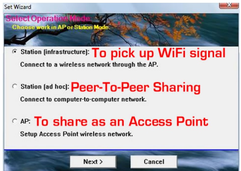
Figure 9 The USB-TurboTenna can be programmed to operate in either as a STATION or an ACCESS POINT mode
